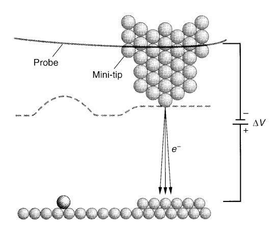
In 1989, IBM scientist Don Eigler (at San Jose, CA) discovered that in addition to using the STM to look at atomic atoms, he could also use the STM as a pair of tweezers to move single atoms! They used the STM to move individual atoms of the gas Xenon that had been cooled to extremely low temperatures so that they sat still, to spell out "IBM" on a nickel surface.
